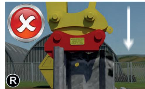
**R** Do not use sudden forces as this could damage the sheet.
