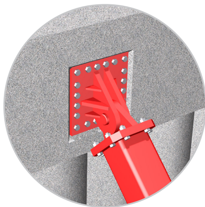
Typical bearing detail on RC capping beam.
